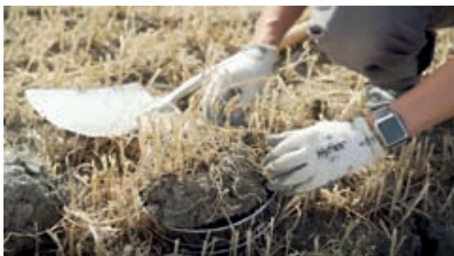
Sampling of undisturbed clod for determination of soil biological quality by microarthropods (QBSar). Photo Arpav
