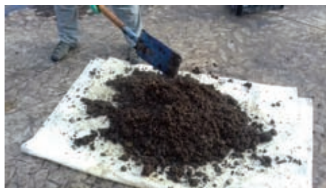
Images of digestate sampling at Brussa biogas plant, Caorle (VE); detail of heap storage of separated solid used as a soil amendment in Agroforcarb experimental site at Vallevicchia and sample collection for analysis. Photo Arpav
